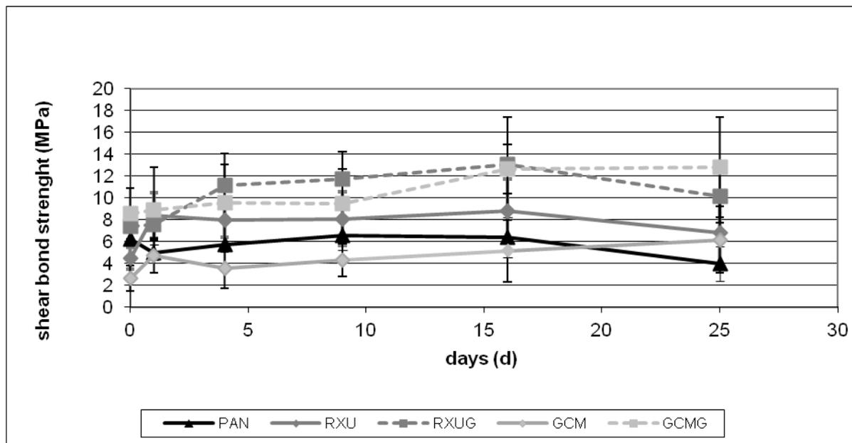
**Figure 4** Diagram of shear bond strength after thermocycling (1, 4, 9, 16, 25 days).
