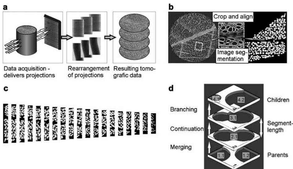
**Figure 1** Schematic workflow (a) and details of the experiments (b–d). (b) Transformation of the selected growth ring in the original cross-section to a binary image; the subset demonstrates the quality of the segmentation method. (c) Binning of a growth ring for porosity measurements. (d) Principle of connectivity analysis.
