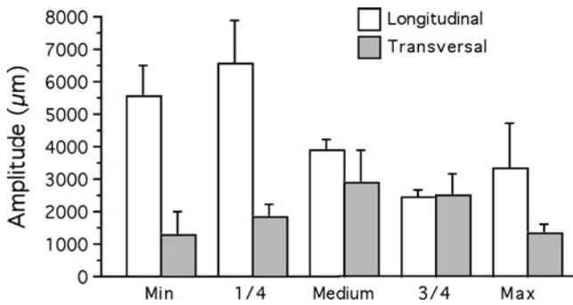
**Fig. 2** Amplitudes of the instrument tip at different power settings
