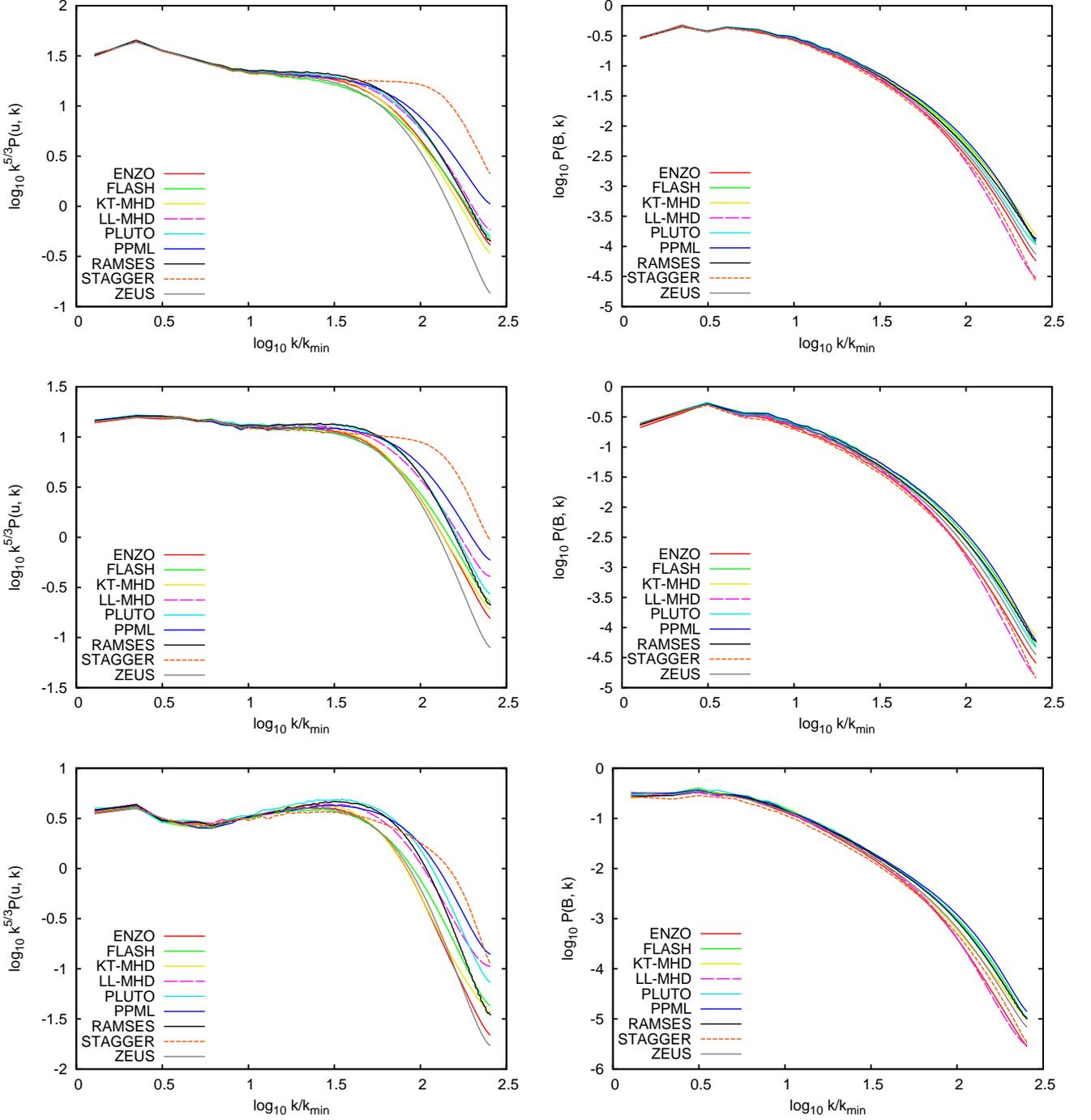
FIG. 3.— Power spectra of the velocity (left panels) and magnetic energy (right panels) on a  $512^3$  grid for flow snapshots 1, 3, and 10 at  $t = 0.02, 0.06,$  and  $0.2$  (top-to-bottom), respectively. The velocity spectra are compensated with  $k^{5/3}$ , while there is no compensation for the magnetic energy spectra. Note that the ordinate scale is not always the same for different time instances.
