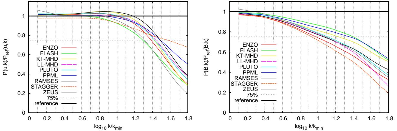
FIG. 4.— Compensated power spectra of the velocity (left panel) and magnetic energy (right panel) for the first flow snapshot at  $t = 0.02$  from the  $512^3$  simulations.
