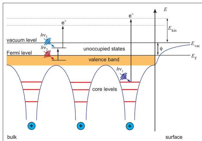
Fig. 1. Core and valence levels at a metal surface that can be probed by photoelectron spectroscopy. One X-ray photon ( $h\nu_1$ ) causes emission of a core electron. Two UV-VIS photons ( $h\nu_2$  and  $h\nu_3$ ) cause emission of a valence band electron via an intermediate state above the Fermi level.
