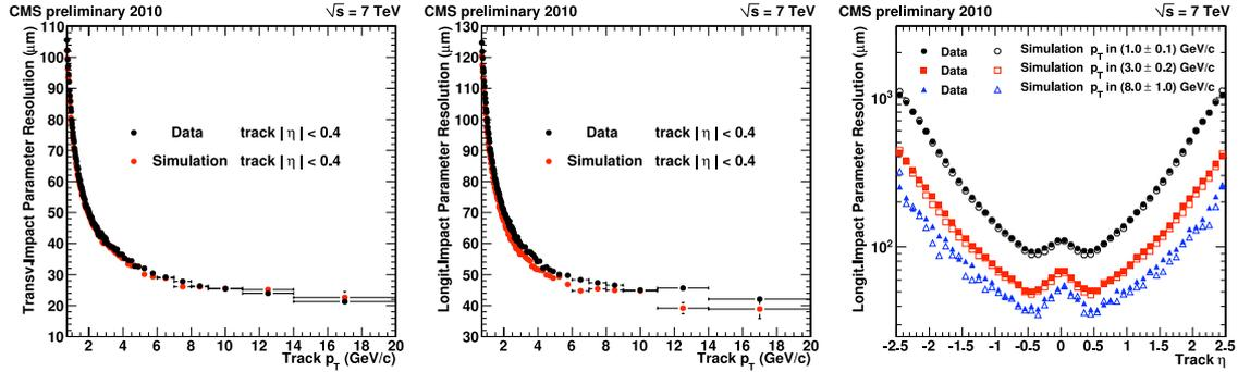
**Figure 3:** Left and middle: The measured resolution of the track transverse and longitudinal impact parameter as a function of track  $p_T$ . Right: The measured longitudinal impact parameter as a function of track- $\eta$ .
