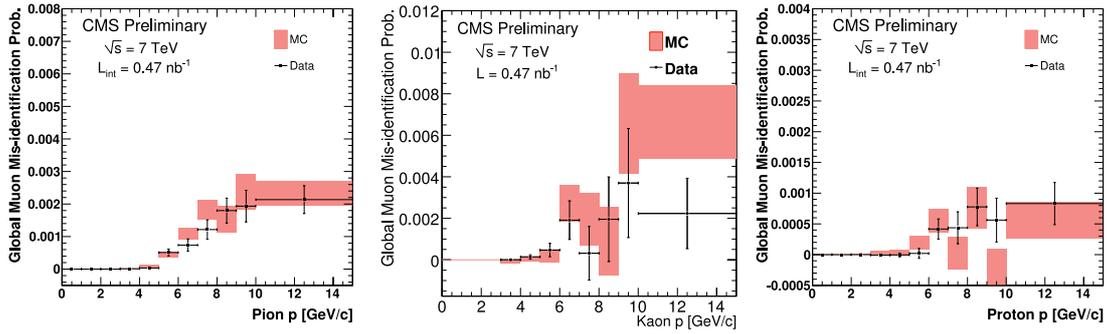
**Figure 7:** The fraction of pions (left), kaons (middle) and protons (right) that are mis-identified as global muons as a function of momentum. The uncertainties that are indicated by error bars (data) and the grey boxes (simulation) are statistical only.
