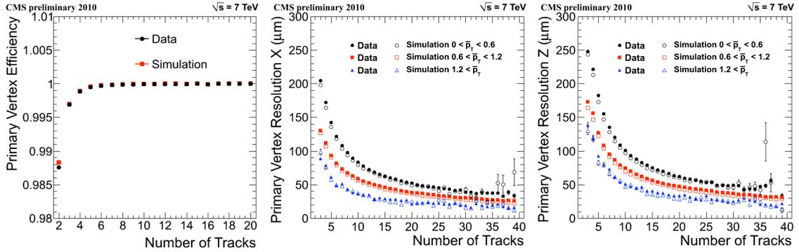
**Figure 2:** Left: The primary vertex reconstruction efficiency as a function of the number of associated tracks. Middle and right: The primary vertex resolution in  $x$  and  $z$  as a function of the number of associated tracks for different average transverse momentum  $\overline{p_T}$ . The Pythia8 Tune1 [5] is used in the simulation.
