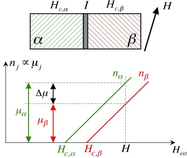
Figure 1: Sketch of an experiment in which two magnetic insulators with different critical fields  $H_{c,j}$  ( $j = \alpha, \beta$ ) are weakly coupled to one another through a magnetically inert spacer layer  $I$  and are placed into an external magnetic field  $H > H_{c,j}$ . The respective condensate densities  $n_j$  and the chemical potentials  $\mu_j$  vary approximately linearly with  $H$ .
