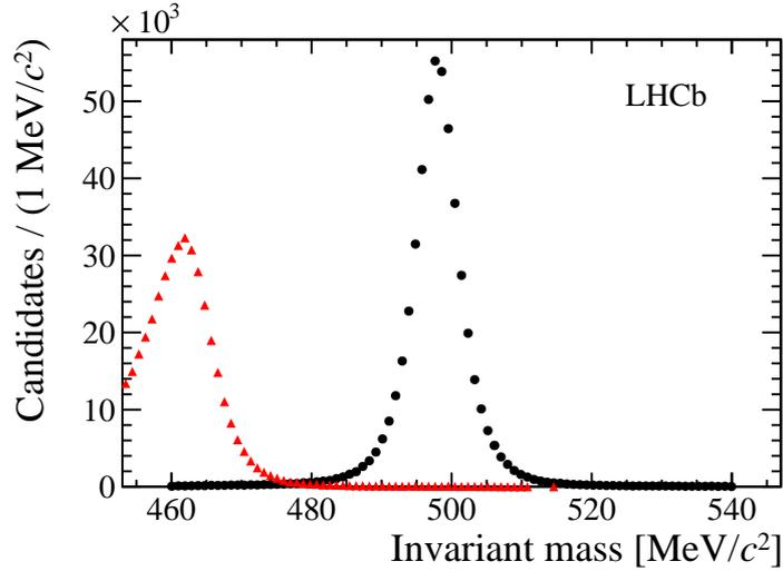
Figure 1: Mass spectrum for selected  $K_s^0 \rightarrow \pi^+\pi^-$  candidates in the MB sample. The black points correspond to the mass reconstructed under the  $\pi\pi$  mass hypothesis for the daughters, while the red triangles correspond to the mass reconstructed under the  $\mu\mu$  mass hypothesis.
