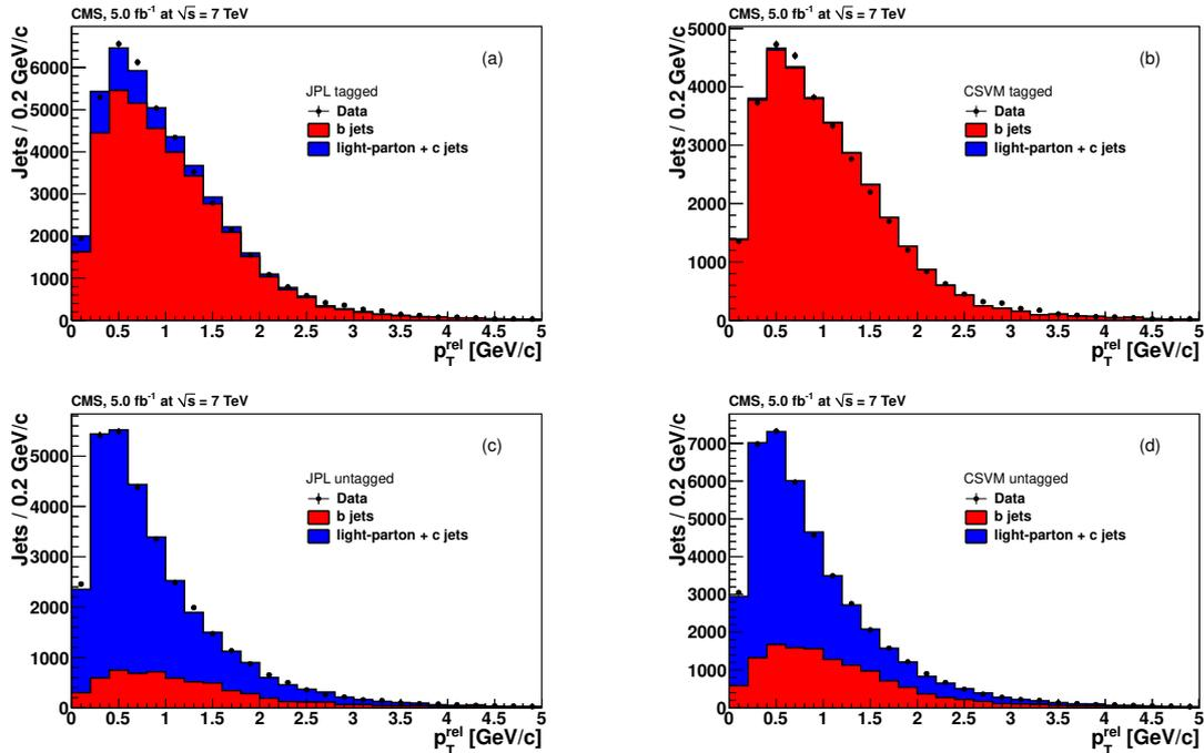
Figure 10: Fits of the summed b and non-b templates, for simulated muon jets, to the muon  $p_T^{\text{rel}}$  distributions from data. (a) and (c) show the results for muon jets that pass (tagged) or fail (untagged) the b-jet tagging criteria of the JPL method, respectively. (b) and (d) are the equivalent plots for the CSVM method. The muon jet  $p_T$  is between 80 and 120 GeV/c.
