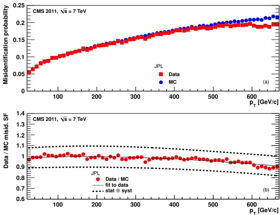
Figure 21: For the JPL tagger: (a) misidentification probability in data (red squares) and simulation (blue dots); (b) scale factor for the misidentification probability. The last  $p_T$  bin in each plot includes all jets with  $p_T > 670$  GeV/c. The solid curve is the result of a polynomial fit to the data points. The dashed curves represent the overall statistical and systematic uncertainties on the measurements.
