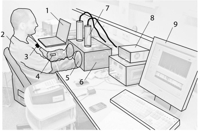
**Fig. 1** Measurement setup. 1: near-infrared spectroscopy (NIRS) data recording, 2: subject, 3: occlusion cuff, 4: attached NIRS device, 5: light shielded opening of the dark chamber to insert the hand, 6: dark chamber, 7: PMT, 8: power supply and PMT controlling electronics, 9: PMT controlling and measurement.
