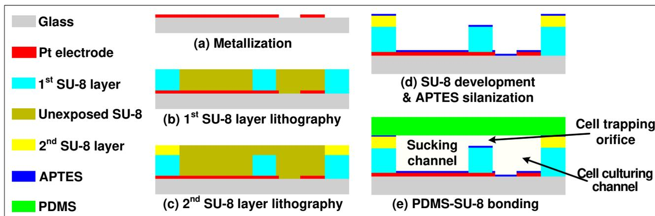
Figure 2: Fabrication process
