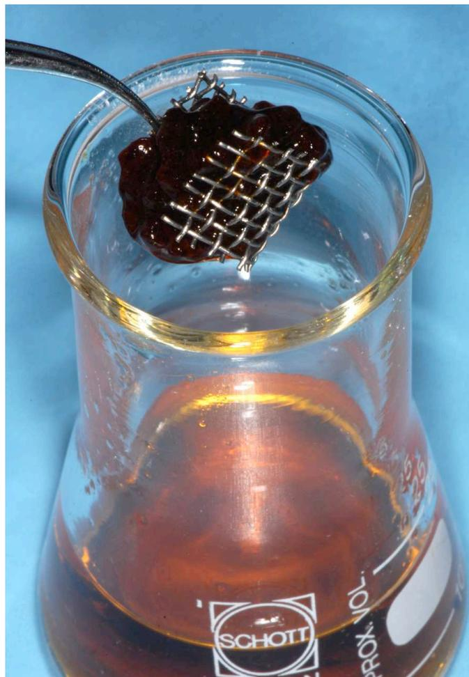
Figure 1: Illustration of the custom-made mesh made of stainless steel, which served for material transfer and stable immersion.
