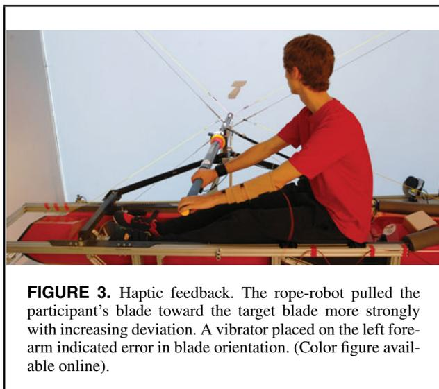
**FIGURE 3.** Haptic feedback. The rope-robot pulled the participant's blade toward the target blade more strongly with increasing deviation. A vibrator placed on the left forearm indicated error in blade orientation. (Color figure available online).
