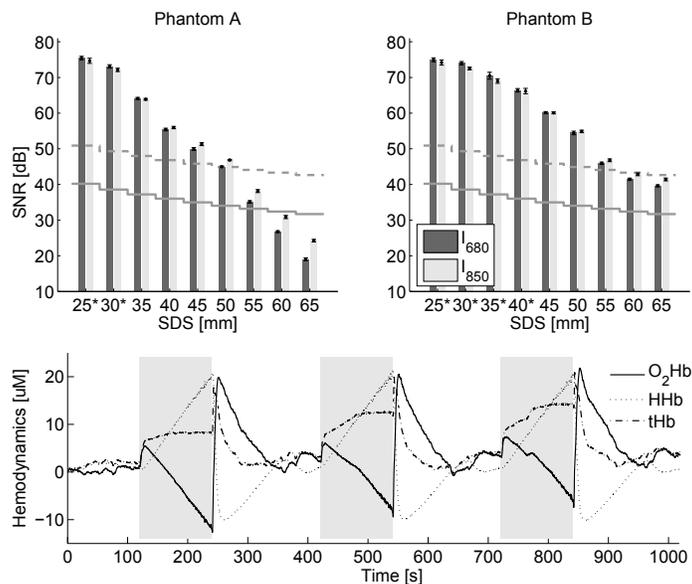
Fig. 2. Top: mean SNR ( $\pm$  SD) vs. SDS, measured at two phantoms (A and B). The dashed (solid) line shows the empirically derived minimal SNR for 680 (850) nm. \*: data from TIA output. Bottom: changes in hemodynamics during three arterial occlusions (gray areas).
