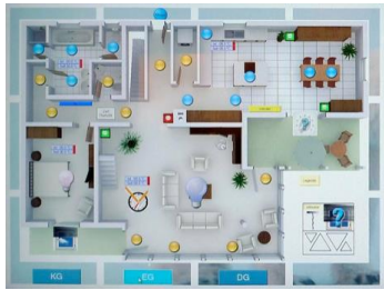
Figure 1: Screenshot of an example of a KNX visualization (EisBär KNX 4 ) using floor plans
