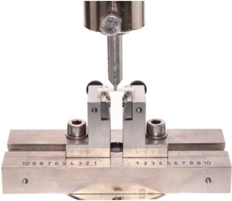
Fig. 2. Sample holder of three-point flexural strength testing method, with a span between the two supports of 12 mm.
